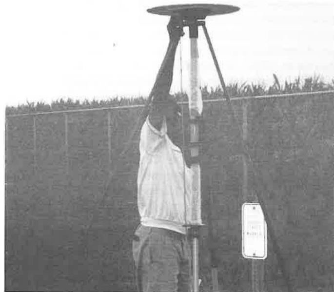
Ed Glass sets up the 2-meter fixed height rod at Mt. Comfort station.
