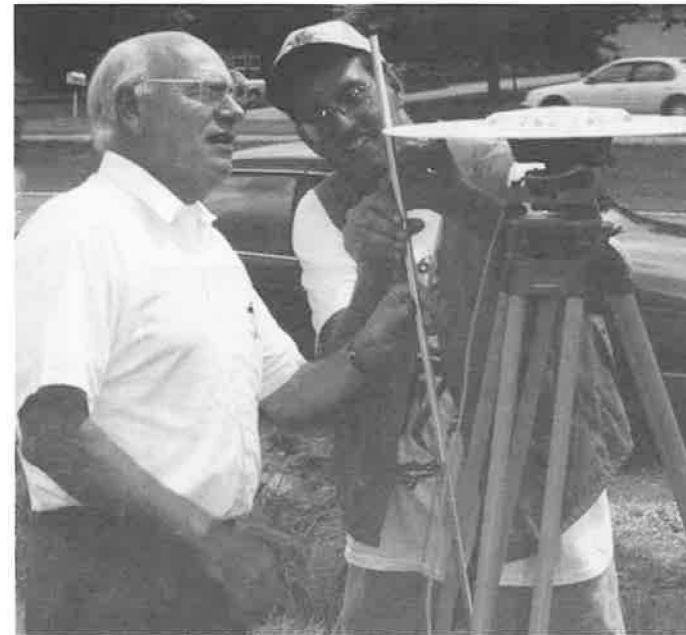
Jack Irwin, P.L.S. Marion County Surveyor and Robert Wilcoxon, Party Chief, measure antenna height at station Mills.
