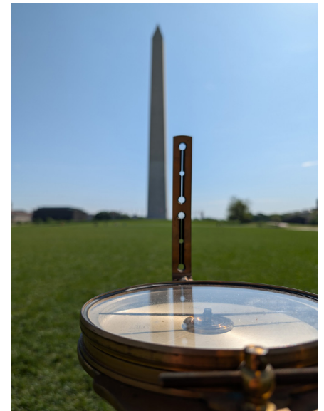
A traverse with a vernier compass and chain was part of the event.
