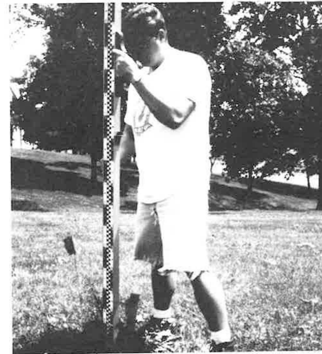
Stephen Pratt concentrates on keeping the level rod vertical during the control surveys.
