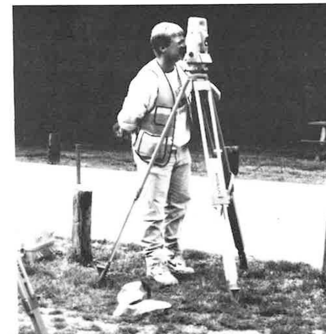
Scott Whybrew takes topo observations with the total station during the Happy Hollow mapping project.
