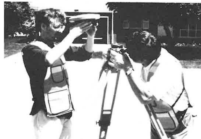
Brent Spencer and Prof. Johnson set up a GPS receiver during the GPS control survey campaign.
