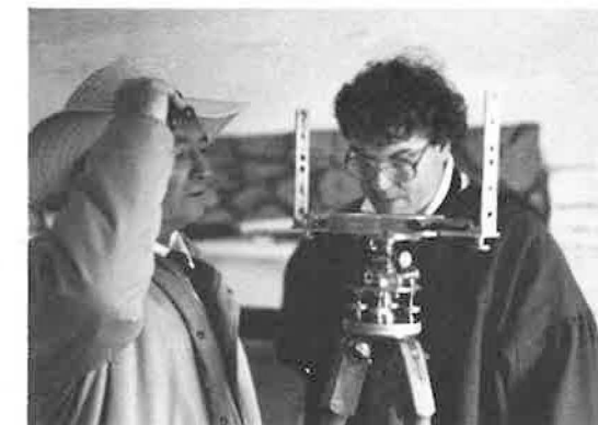
Hal Ashton of Middletown and Robert Cottrell of Conner Prairie viewing an Andrew McNeely (1802-1851) vernier compass with peep sights. Photo taken in the schoolhouse.
