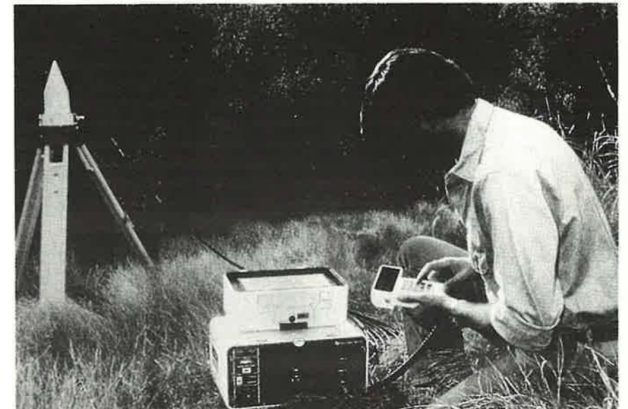
■ GLOBAL Positioning Satellite receiver system consists of a radio receiver and antenna assembly, precise timing device, and a system for recording radio signals.
