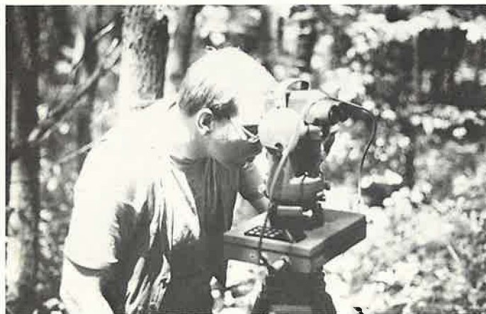
Deep in the woods, a student uses a Wild T-1 theodolite and DI-3S distomat in measuring a traverse to bring state plane coordinates to new stations from existing horizontal control in the area.
