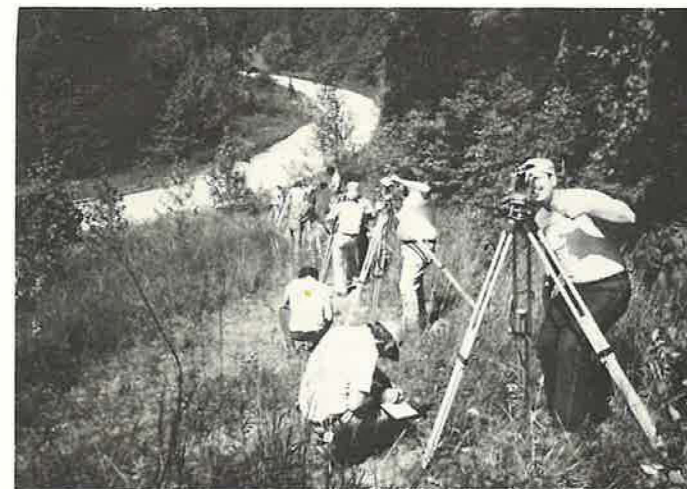
Several primary and secondary control traverses were run throughout the area. Solar observations for azimuth checks were made to verify results.
