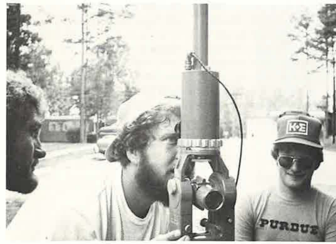
Students also had the good fortune to use the Wild gyrotheodolite (shown above) and the K & E Vectron electronic theodolite and data collector, due to generosity of Wild (Mike Kaminski) and K & E (Dennis Middleton).
