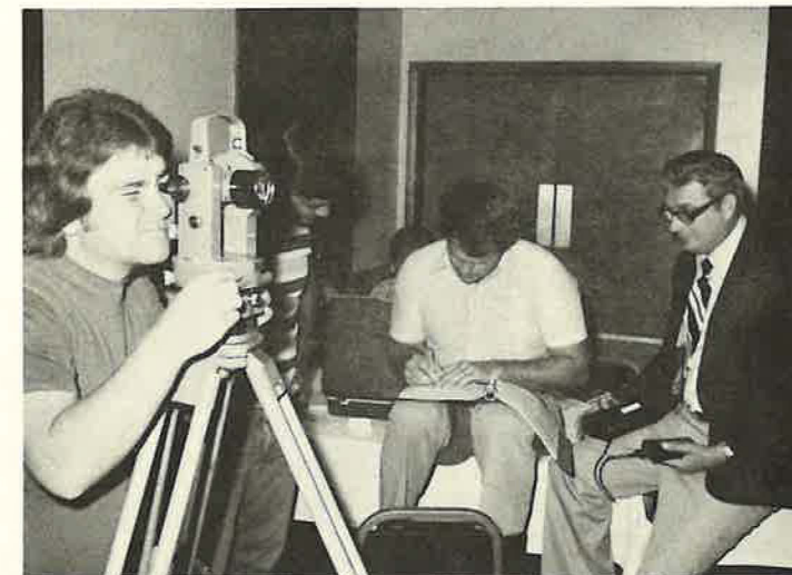
After taking a number of readings with theodolites having optical micrometer coincidence knobs, the reading and pointing errors were analysed with respect to precision. Topics discussed included the nature of measurement, systematic and random errors, precision, mistakes, specifications, standards, and care of instruments.
