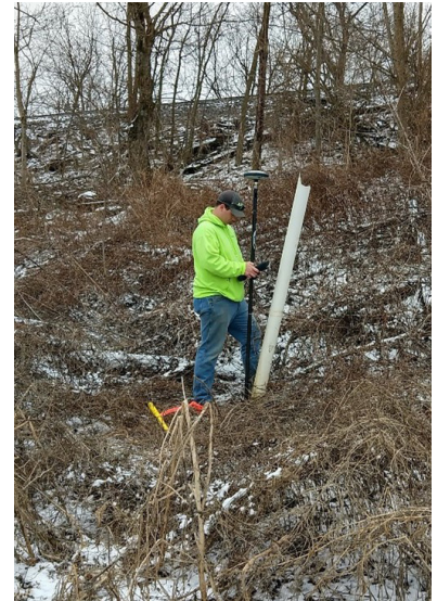
Luke Strotman locating possible corner monumentation.
