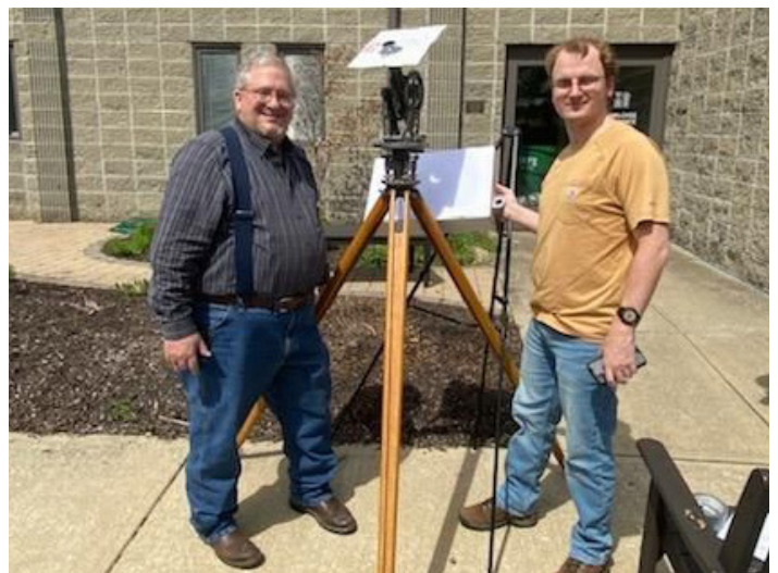
ISPLS Past-President Vince Barr and Nick Coyle show a sun shield atop a transit at VS Engineering that made the sun's image more visible during the solar eclipse. Both are in the Right-of-Way Engineering Department.
