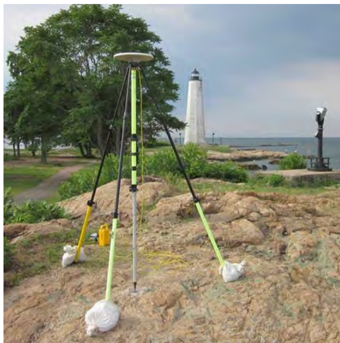
Figure 5: An example of GPS equipment setups on a bench mark
