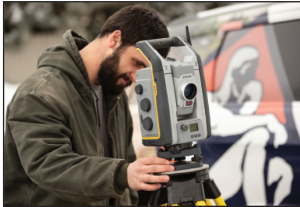
Aaron Bender, surveying technician, sets up the and land development instrument to begin a new survey project.
