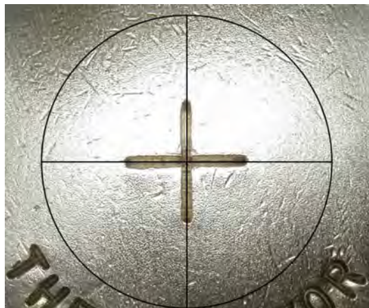
Magnification possible from the Wild Model NL optical plummet.
