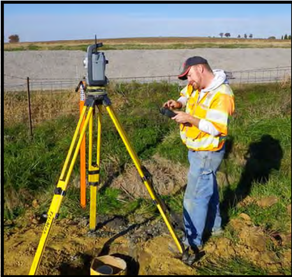
Matt Badger multi-tasking while making an observation with the Trimble S8 High Precision Total Station.
