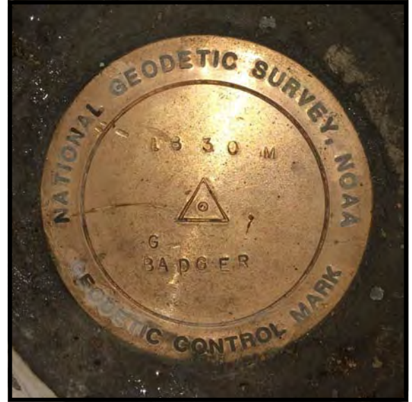
One of the four Geodetic Control Marks. The station was named "G BADGER" in honor of Matt's father and set at 1,830 meters along the base line. Photos provided by Matt Badger.
