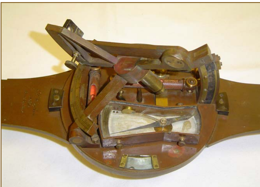
This view of the Hougham Solar Compass at the Johnson County Museum shows the compass needle box and the detailed components used in conjunction with the sun's rays to align the compass to true north and measure the deflection of the needle. An engraving on the plate at left reads "J.S. Hougham, Maker, Franklin, Ind."
