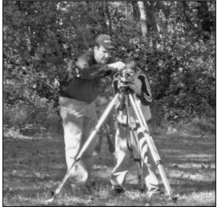
Scout Darien Mattix receives pointers from merit badge counselor Aaron Blank, PLS, on how to focus the level on the rod held just out of the photo by fellow Scout Matt Lewis.
