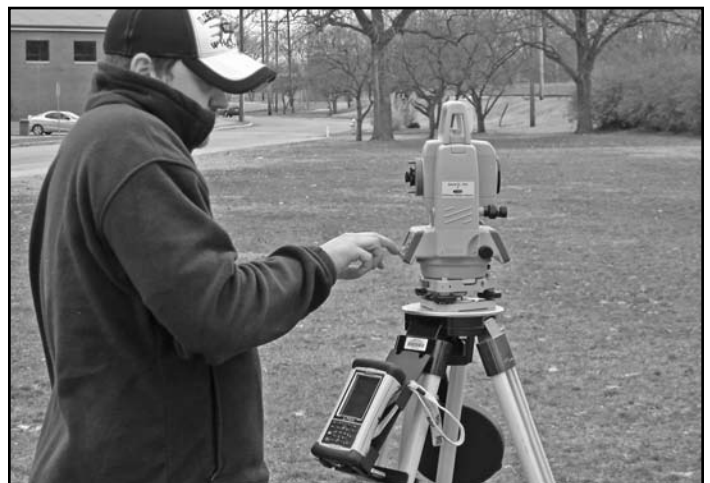
V.U. Land Surveying Technology student, Jedadiah Mullen traversing with the new Topcon equipment
