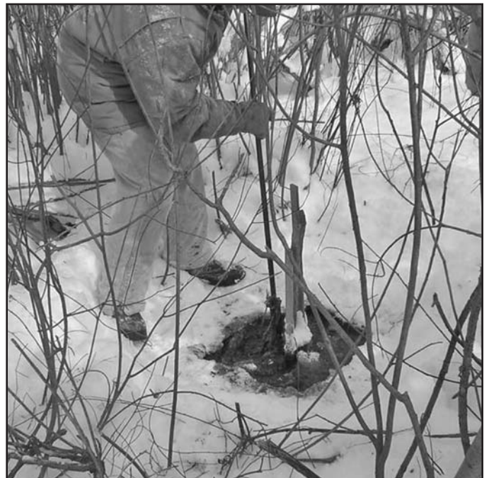
Tom Stephenson, PS, of Cassopolis Mich., uses an ice-fisherman's spud bar to open a hole in the ice on the surface of a swamp at mile point 52 on the Indiana-Michigan state line, where three years ago he located an original 1827 post set by U.S. District Surveyor Eleazer P. Kendrick.
