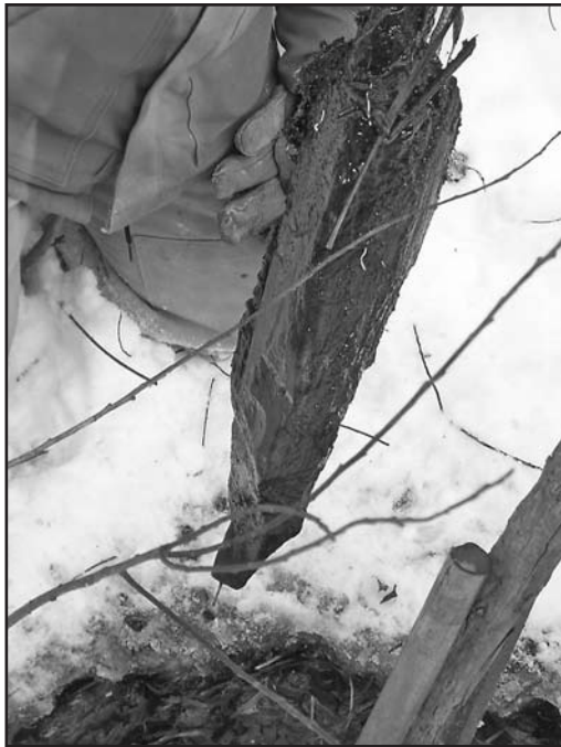
Tom Stephenson, PS, of Cassopolis, Mich., holds remnants of mile post 52 pulled from the waters of a swamp on the Indiana-Michigan boundary about three miles north of Bristol, Ind. When he first located the post's position in January 2004, the piece of cedar at lower right in the picture was the only evidence above the surface. He found the mile post under the icy water and then marked the location with the three-quarter-inch pipe shown alongside the cedar "stick."
